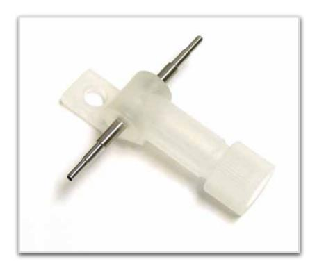
Bubbles in HPLC systems can cause check valve malfunctions and pump cavitation, seriously affecting pump performance. A Debubbler is a small reservoir designed to remove bubbles from the inlet fluid stream of the pump.
